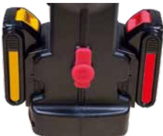
5) Slide the battery cartridge into adaptors making sure the battery pack is fully seated.
