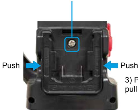
3) Push here on both sides and pull off the adaptor.
